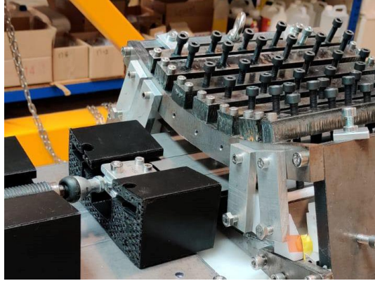
Figure 5: sliding process of the magnets during the assembly
