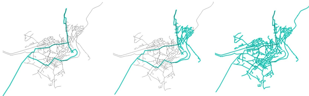
Figure 2 Iterative topological analysis: pipes connected to water sources (cyan); WDN layout from water utilities’ database (black).
