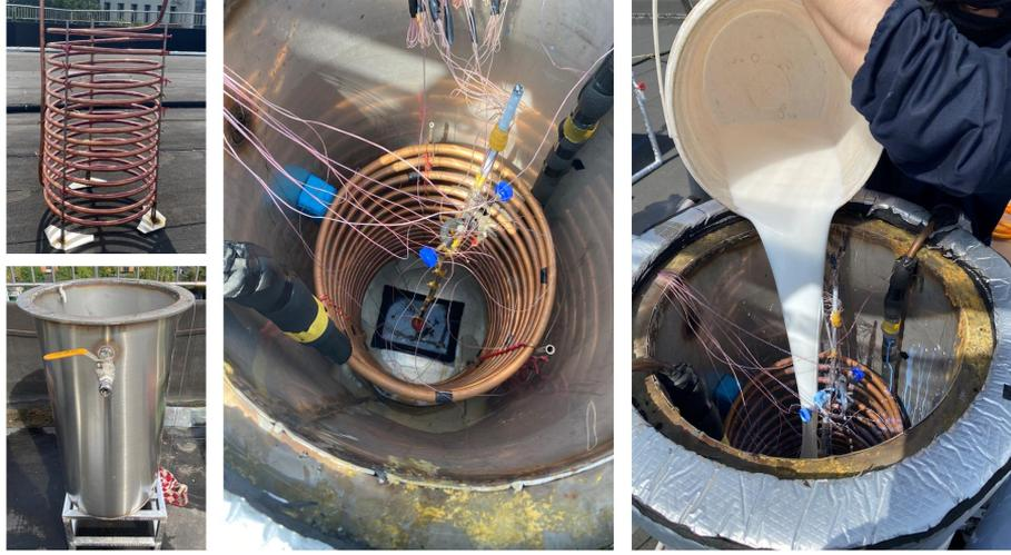
**Figure 1c:** Physical diagram of evaporative heat accumulator.
