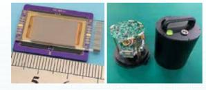
MEMS Accelerometer and Seismometer
