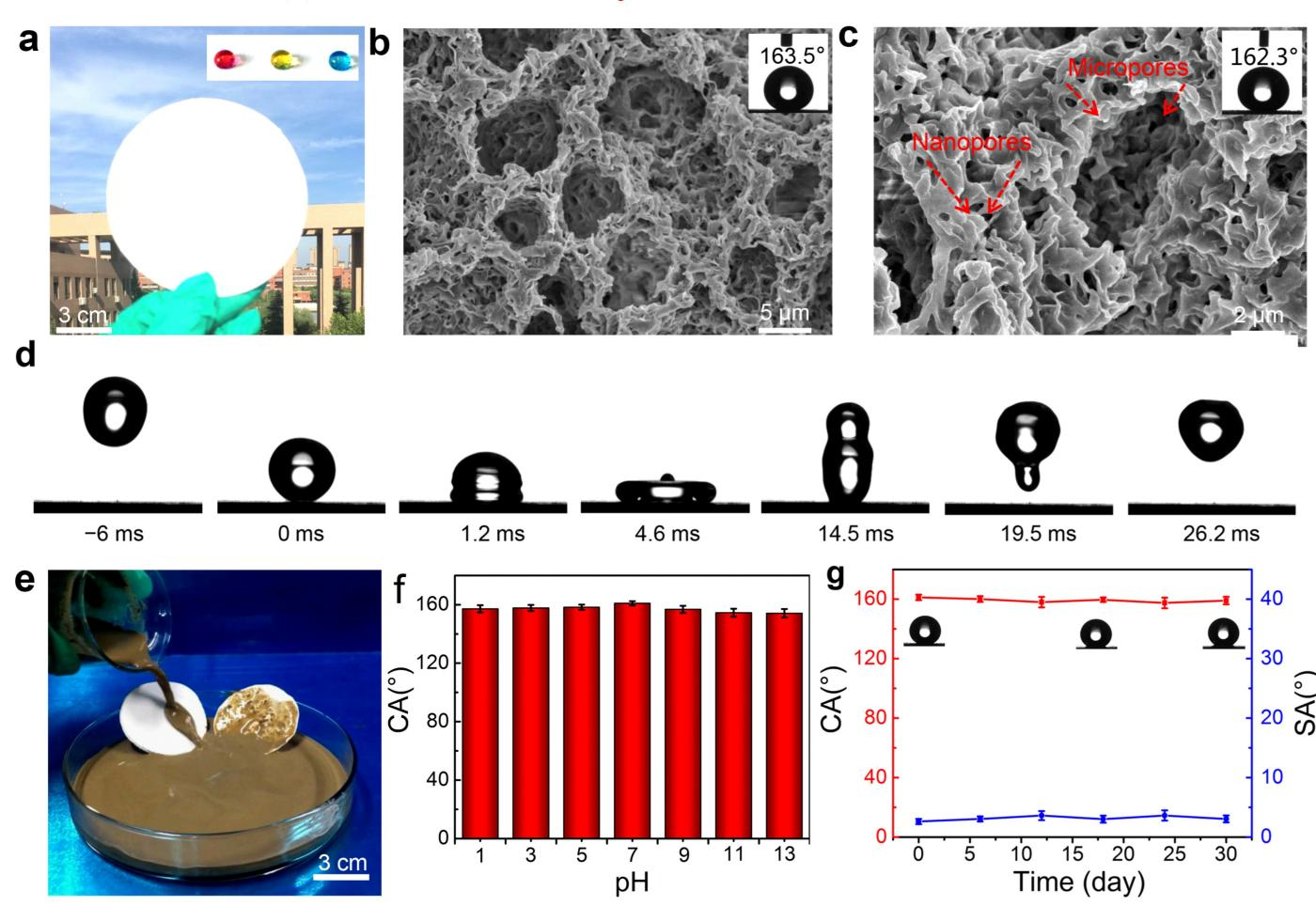
The superhydrophobic radiative cooling porous (SRCP) film shows an ultra white appearance and has excellent super-hydrophobic properties.
