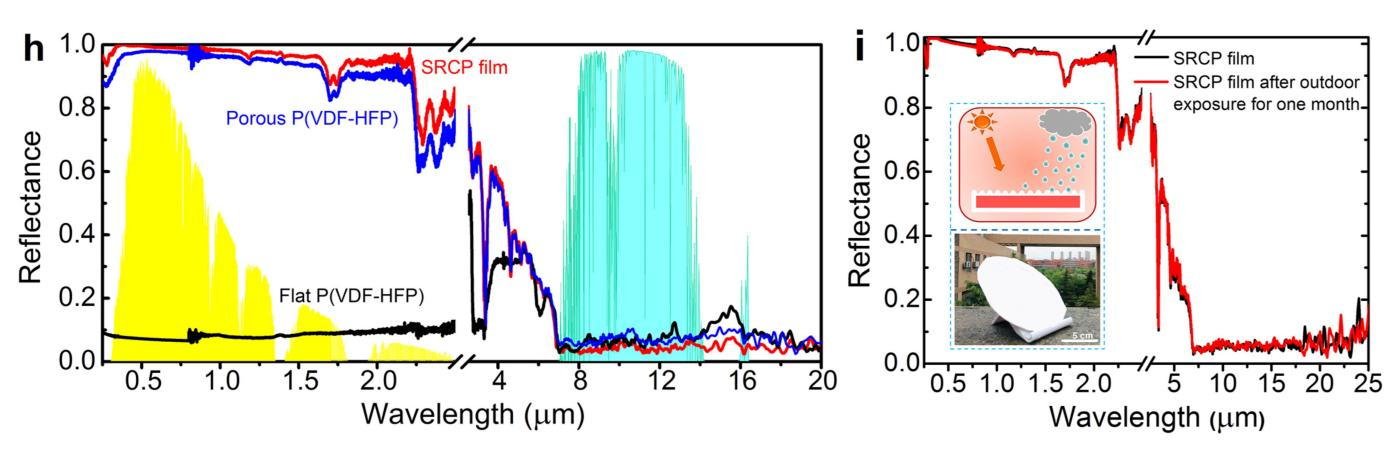
The SRCP film surface has a high sun reflectance to minimize absorption heat from sun and high thermal infrared emittance to favor sending heat loss to the sky.
