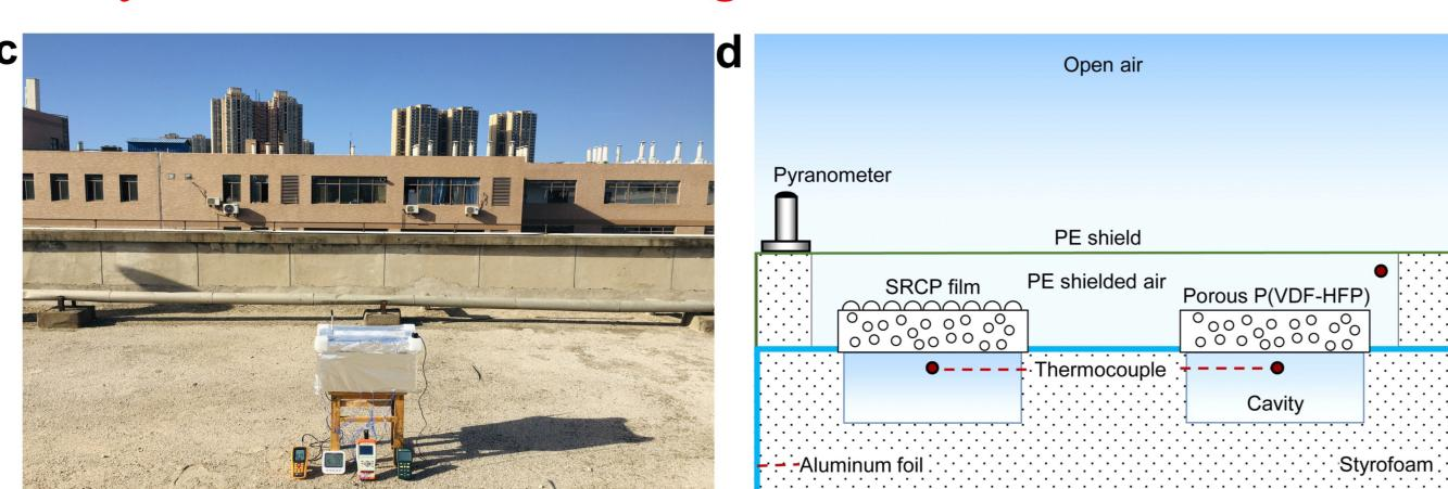
The photo of the cooling setup on the rooftop and its illustration.
