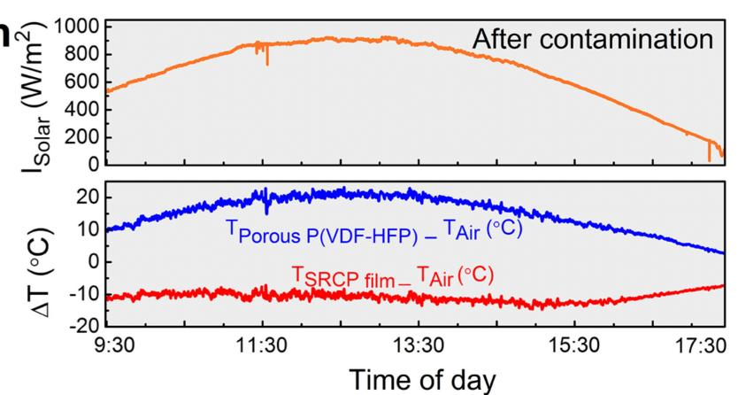
When the SRCP film was exposed to the environment, its temperature dropped to approximately 13.8 °C below the air temperature. In contrast, the porous P(VDF-HFP) film was prone to mud contamination and its surface temperature dramatically rose to 20.6°C above the ambient temperature.
