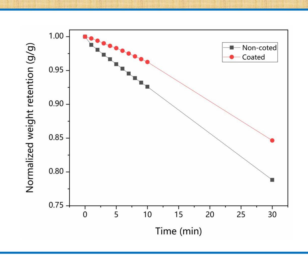
Water molecules are distributed in the hydrogel network. However, water will be inevitably evaporating at the interface with air. The covalent binding hydrophobic polymer wrap the hydrogel surface, act like stratum corneum in skin. It takes ~twice time in coated sample than non-coated sample to evaporate the water of same weight.
