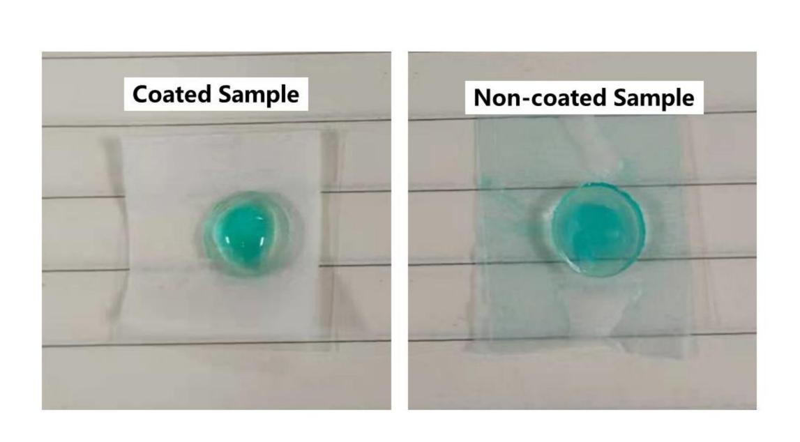
After surface modification, the substance release can be site controlled. A drop of CuSO<sub>4</sub> solution was added onto the surface of hydrogel. Non-coated sample will be infiltrated rapidly, and the dry paper was dyed to be blue. Whereas, the paper under the coated sample keep clean.
