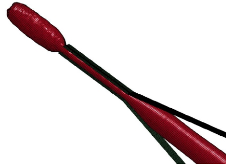
图7 软体通过缝隙的仿真结果 Fig.7 Simulation results of airbag passing through the gap
