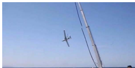
图 3 “天钩”(Skyhook)回收系统 Fig. 3 Skyhook recycling system
