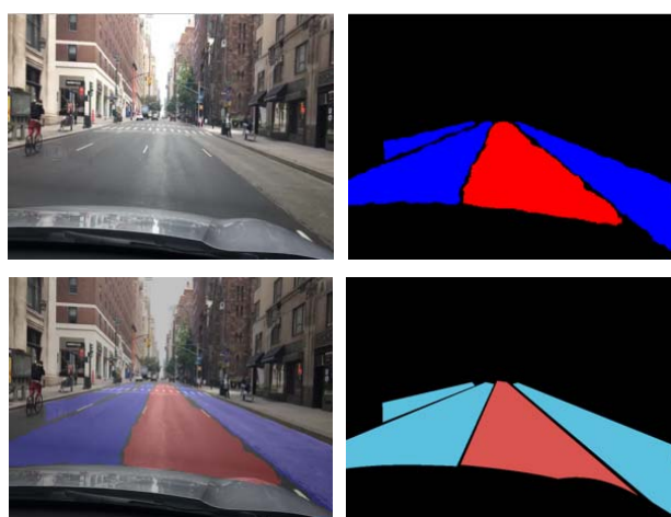
图10 街道可行驶区域图像语义分割结果 Fig. 10 Semantic segmentation results of street drivable area
