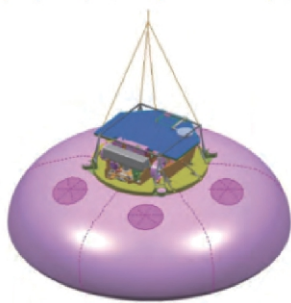
图8 ExoMars采用的组合式气囊 Fig.8 The modular airbag used by ExoMars
