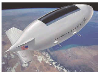
图9 美国的高空无人飞艇HAA Fig.9 High altitude unmanned airship HAA of the United States
