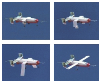
图12 Dryden I2000充气机翼无人机飞行部署过程 Fig.12 In-flight deployment sequence of Dryden I2000 inflatable wing aircraft
