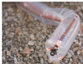
图16 仿藤蔓自生长软体充气式机器人 Fig.16 Vine-like self-growing soft inflatable robot
