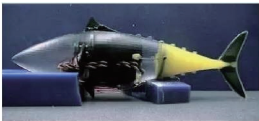
图3 仿金枪鱼潜航器实物图 Fig.3 Real object of biomimetic tuna unmanned underwater vehicle
