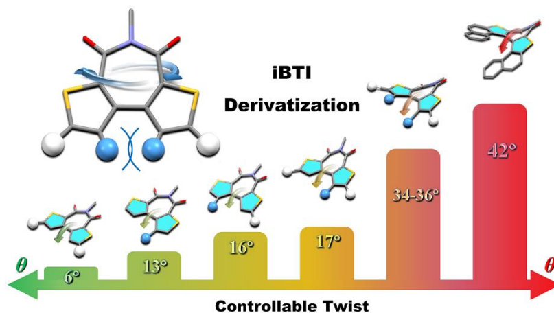
Fig. 1 The torsion angle of the iBTI backbone increases with the number of \beta -position substituents.
