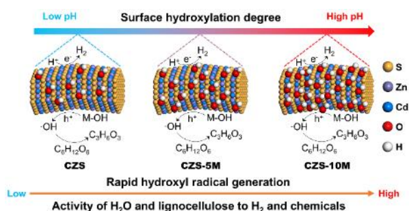
Fig. 1 Schematic of the pH-triggered hydroxylation-hydroxyl radical-photoactivity in the lignocellulose photoreforming.
