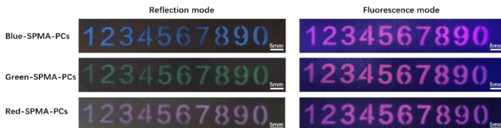
Figure 7. Photos of PCs: reflection mode on the left and fluorescence mode on the right.
