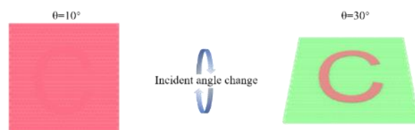
Figure 1 Patterning principle of multi-angle patterned photonic crystal film
