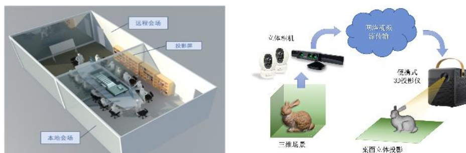
Fig. 1 Schematic diagrams of the remote display and interaction system for online education based on stereo projection. Left: Remote conference room based on large screen stereo projection. Right: Small-scale stereo display system based on desktop stereo projection.
