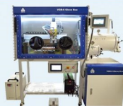
SP-MSM360 32- Cavity High-Throughput Arc Melting System
