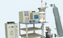
Induction Melting Furnace
