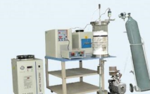
Induction Melting Furnace
